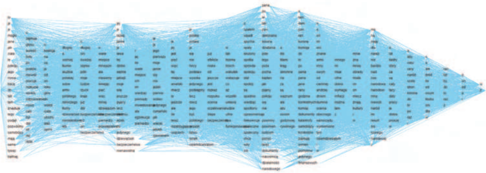
Fig. 5. Real word lattice generated by AGH ASR system shows complexity of the graph and importance of applying language modelling like n-grams
