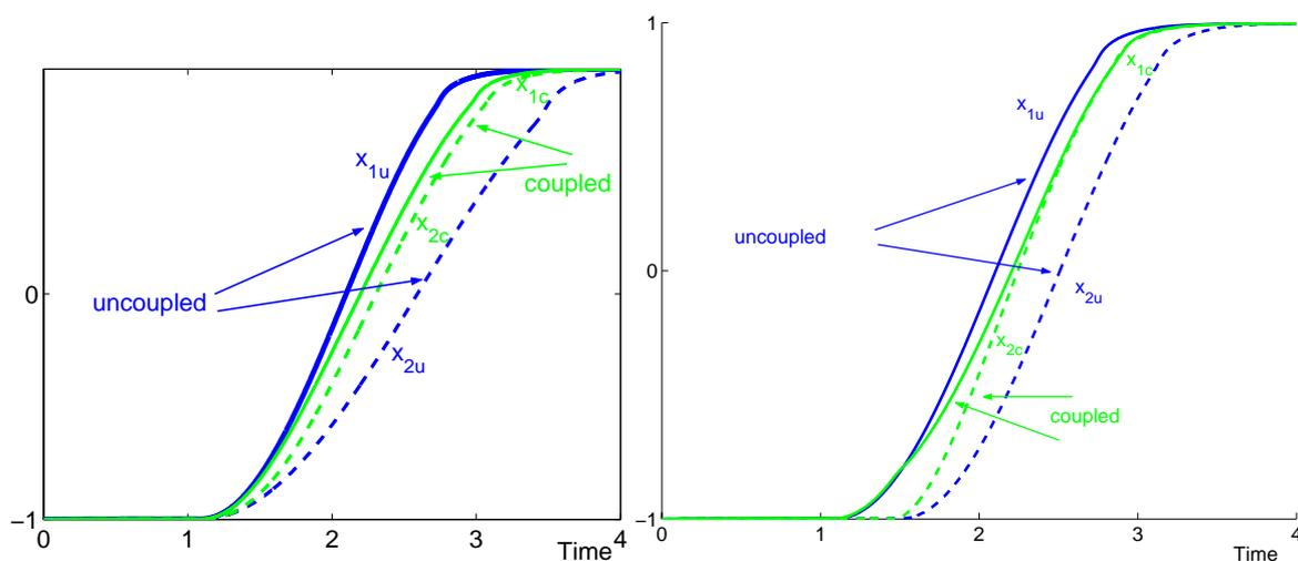
Figure 6. a) Coordination between two timing dynamics through coupling leads to synchronization when movement times differ (2 vs. 3). b) Movement initiation is slightly asynchronous  $t_{init1} = 1$  and  $t_{init2} = 1.4s$  ( $\Delta t_{init} = 5\%$  of MT),  $MT_1 = MT_2 = 2s$  and  $c = 1$ )
