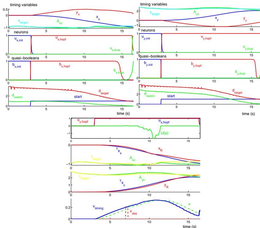
Figure 8. Time courses of variables and parameters for the robot trajectory depicted in Figure 7. Top panels depict timing and neural dynamics ( $x$  and  $y$  coordinate in left and right panels, respectively). Bottom panel depicts neural and timing variables, robot trajectories, real target locations, periodic motion amplitudes and velocity variables.
