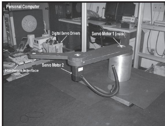
Fig. 1. Planar Manipulator of 2-DOF.
