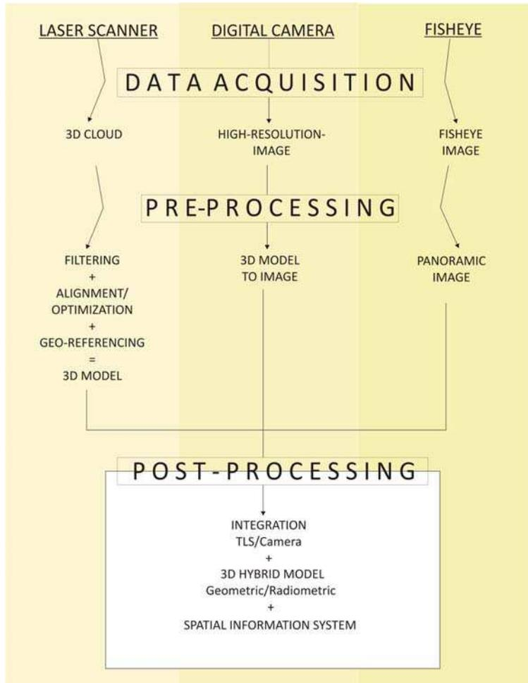
Fig. 1. Methodology for the non-destructive techniques developed and practiced in caves with Palaeolithic art in the eastern part of Asturias (Spain).
