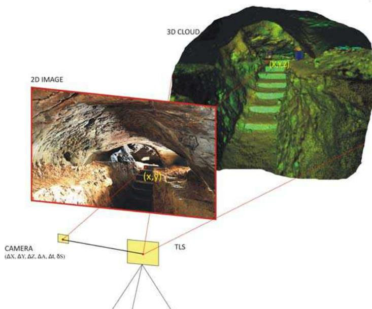
Fig. 4. Registry of the laser scanner and digital camera
