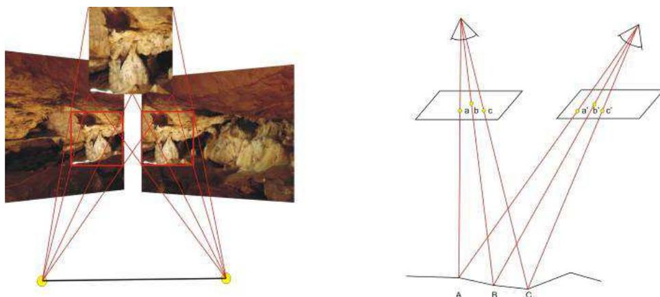
Fig. 3. Left: Principle of the stereoscopic pair. The visualization of the left image by the left eye alone and of the right image by the right eye alone leads to the plastic display of the photographed object. Right: Principle of the "floating mark": the left and right marks are interposed in the optical path of the left and right eye, leading to the perception of a single mark that runs the depth of the object, that is, the mark "floats".
