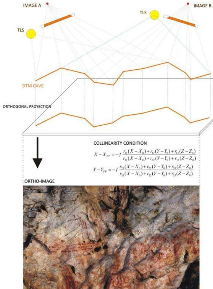
Fig. 5. Orthorectification process and orthophoto generated on a prehistoric panel description of the importance of the each cave is provided remarking the main Palaeolithic art of each cave. Furthermore, from a technical point of view, a brief comment about the constraints of each case of study and the way they have been solved is discussed.
