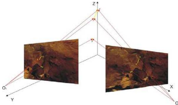
Fig. 2. The object can be reconstructed from the reconstruction of homologous perspective rays (direct intersection).
