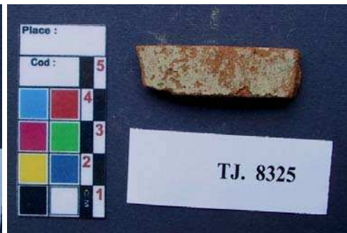
Fig. 4. Salt recrystallization on the surface through capillary effect of high porosity ceramics.
