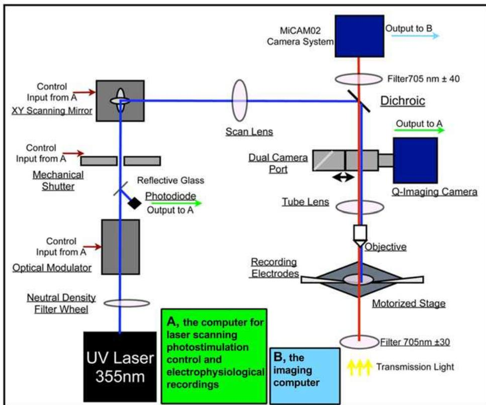
Fig. 1. The general system design for combining laser scanning photostimulation (LSPS) with voltage sensitive dye (VSD) imaging. The diagram shows the whole system consisting of laser scanning photostimulation, VSD imaging, and electrophysiological recording systems. This figure was modified from Xu et al. (2010) with permission of the American Physiological Society.
