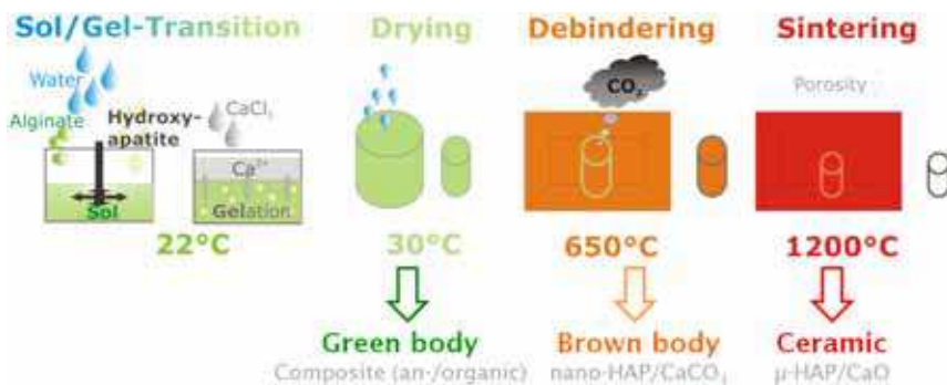
Fig. 7. Sketch of ceramic processing using sol-gel-technique of ionotropic gelation of alginate slurries with ceramic powders
