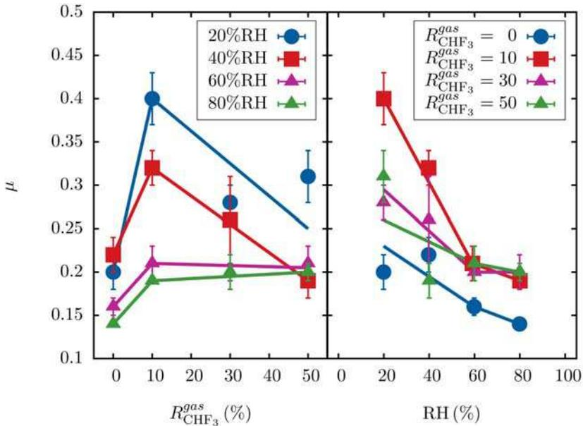
Fig. 6. Friction dependence on humidity and fluorination degree.
