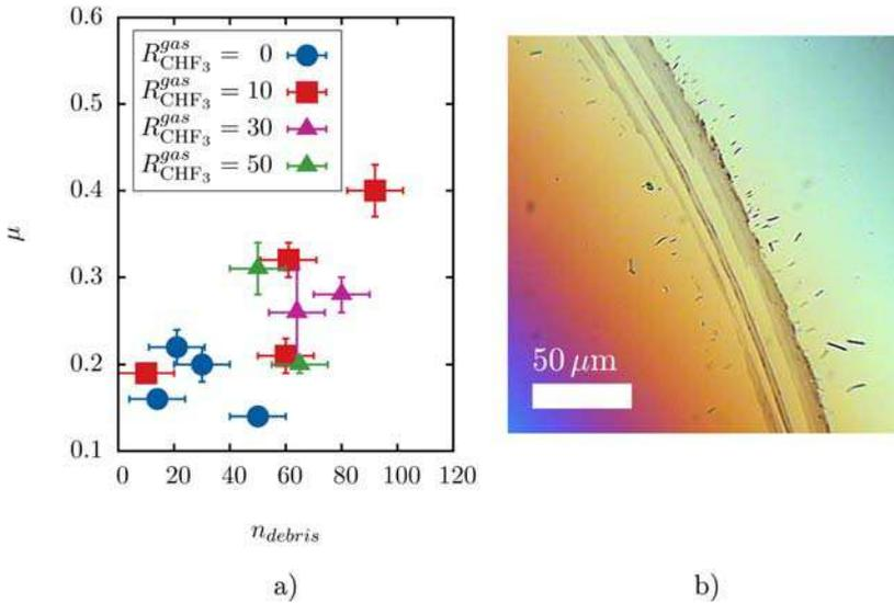
Fig. 5. a) Friction vs number of debris particles visible at  $50\times$  ( $200\times 200 \mu m$ ). The dependence of friction with number of particles is only clear for high friction values; b)  $50\times$  optical microscope picture of a typical sliding track, corresponding to a film with  $R_{CHF_3}^{gas} = 10\%$  measured  $CHF_3$  at 60% RH. Fiber-like debris particles are present at both sides of the sliding track.
