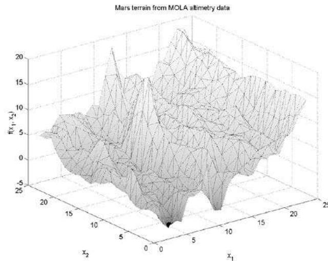
Fig.10. Mars terrain after Delaunay triangulation.
