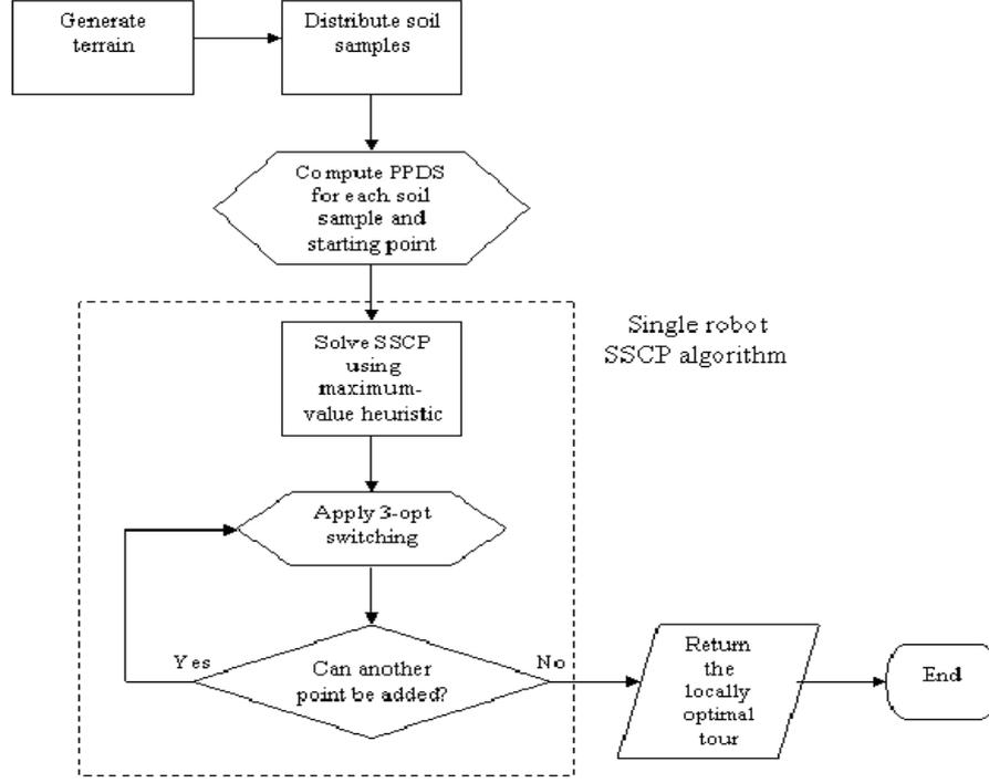
Fig. 2. Flow chart for the single rover case.
