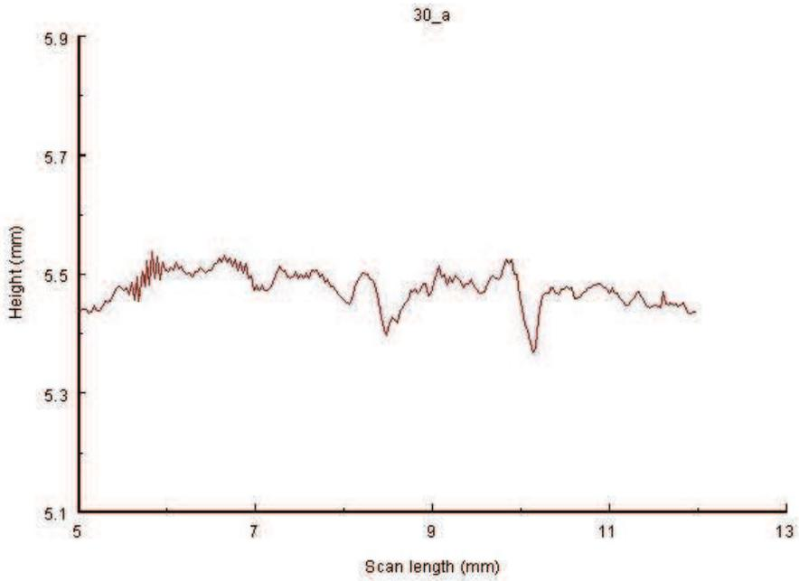
Fig. 4a. 30 micron scan from polished aggregate surface
