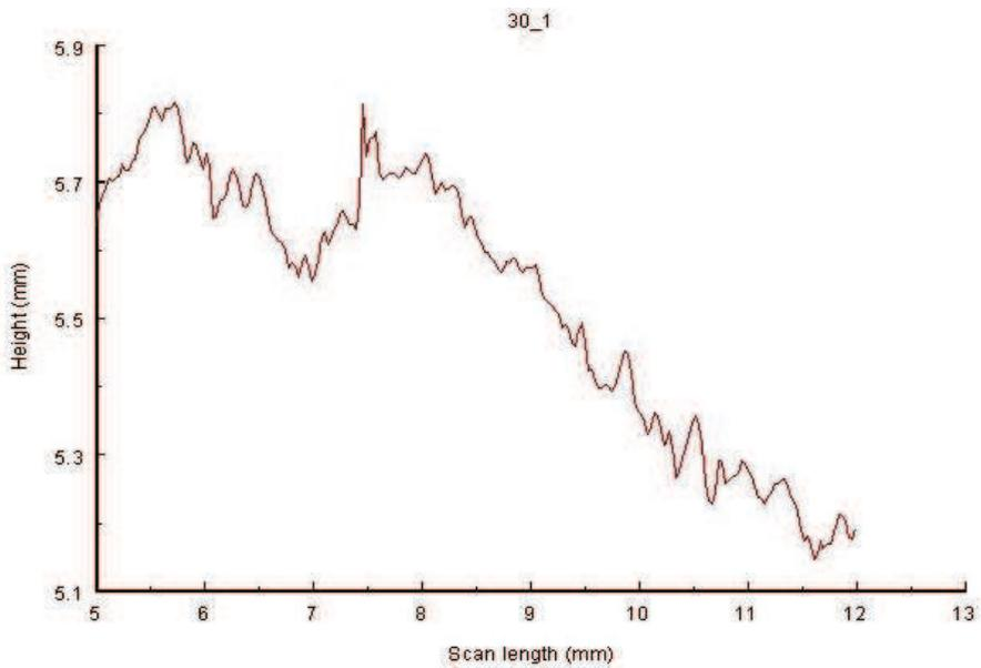
Fig. 4b. 30 micron scan from unpolished aggregate surface
