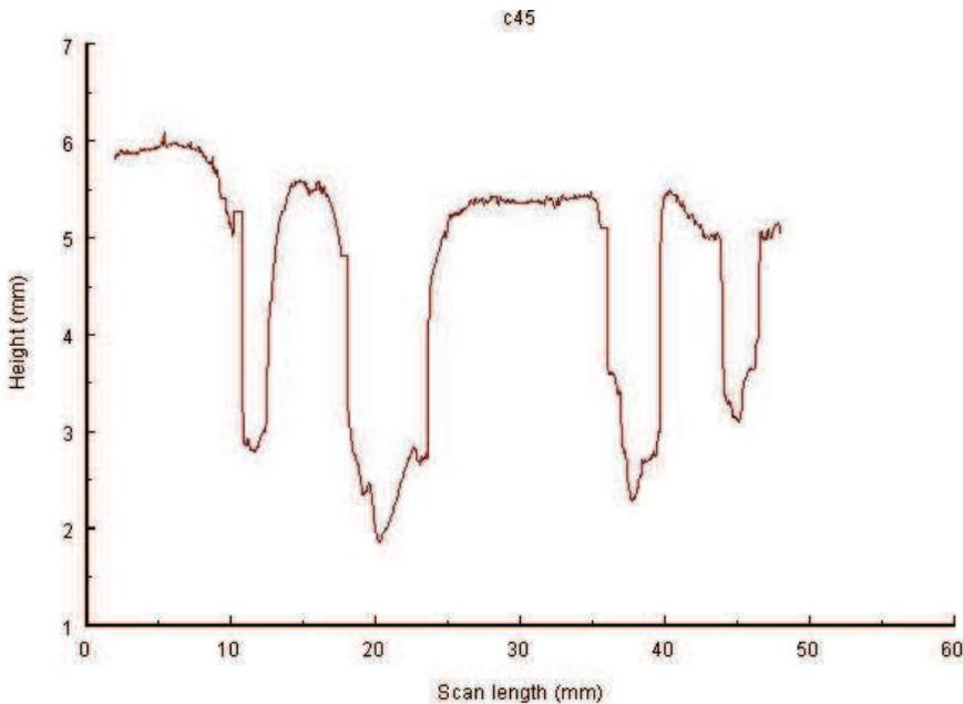
Fig. 5a. 45 micron scan from polished aggregate surface
