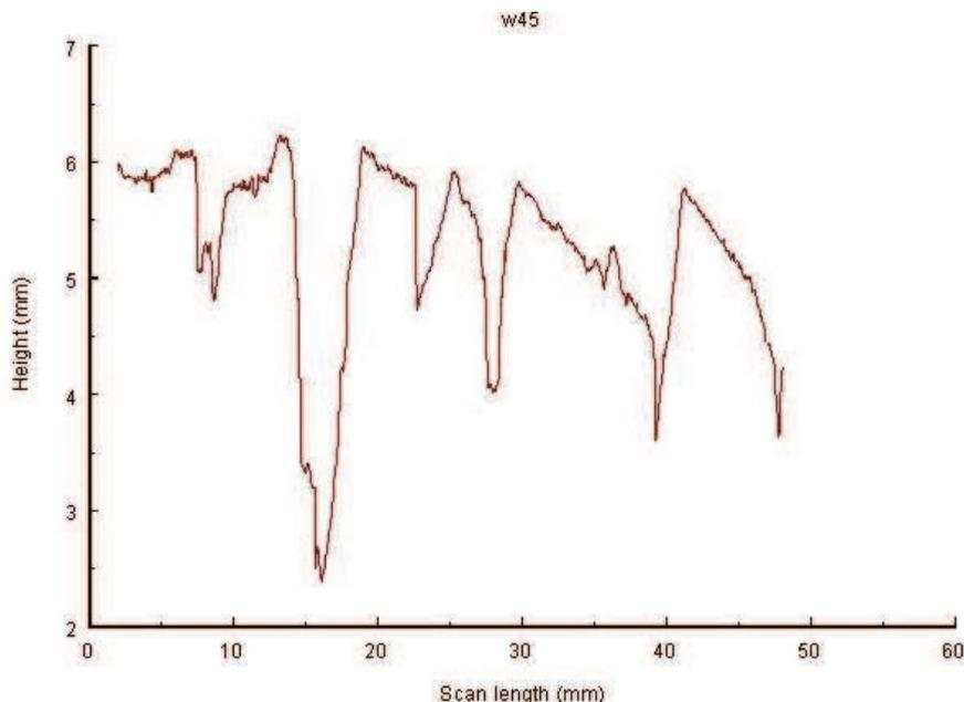
Fig. 5b. 45 micron scan from unpolished aggregate surface
