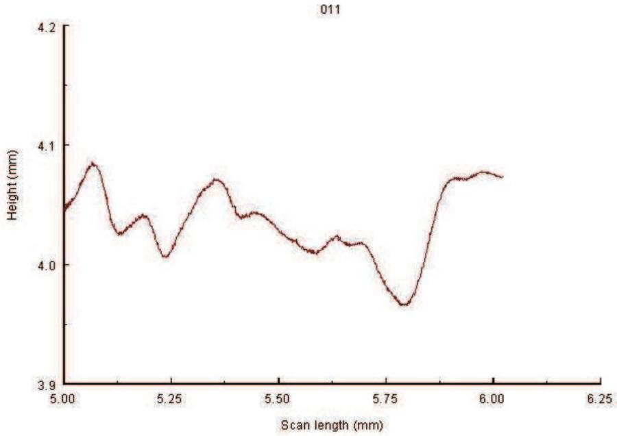
Fig. 2a. 1 micron scan from polished aggregate surface
