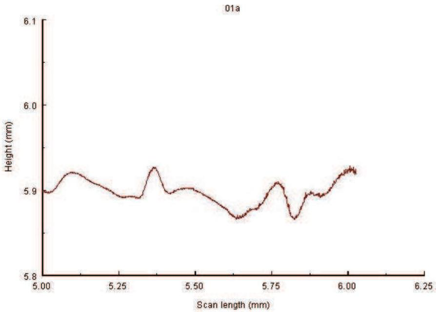
Fig. 2b. 1 micron scan from unpolished aggregate surface
