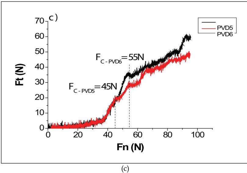
Fig. 12. Scratch-tests carried out on the multi-layers:
