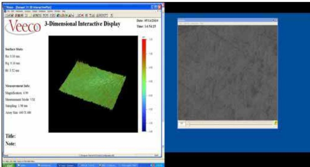
Fig. 1. Topography of coating PVD<sub>1</sub> obtained by the optical profilometer.
