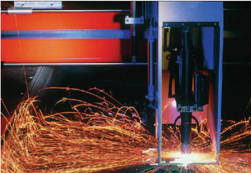
Fig. 2. Plasma cutting process for metal plates
