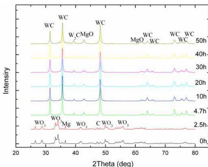
Fig. 1. The XRD patterns of the mixed powders after milling for different time
