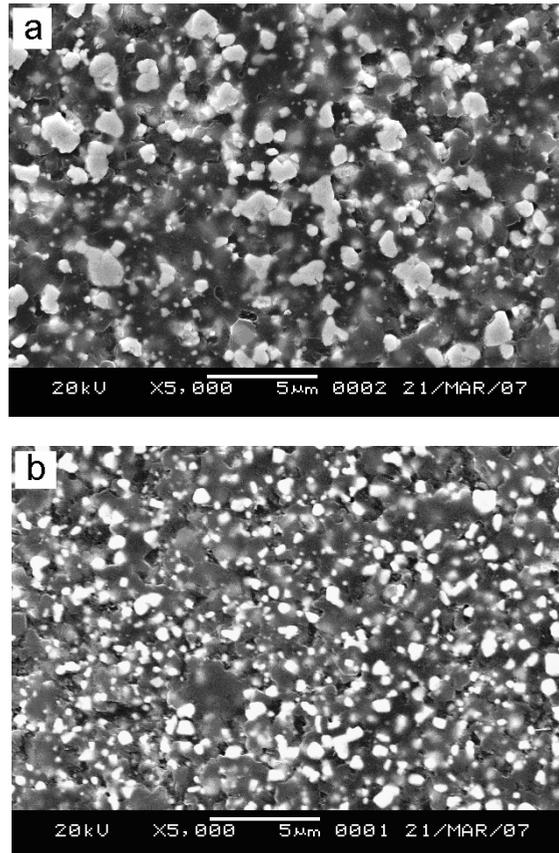
Fig. 14. Backscattered micrographs of polished surfaces of the samples sintered by (a) HPS and (b) PAS
