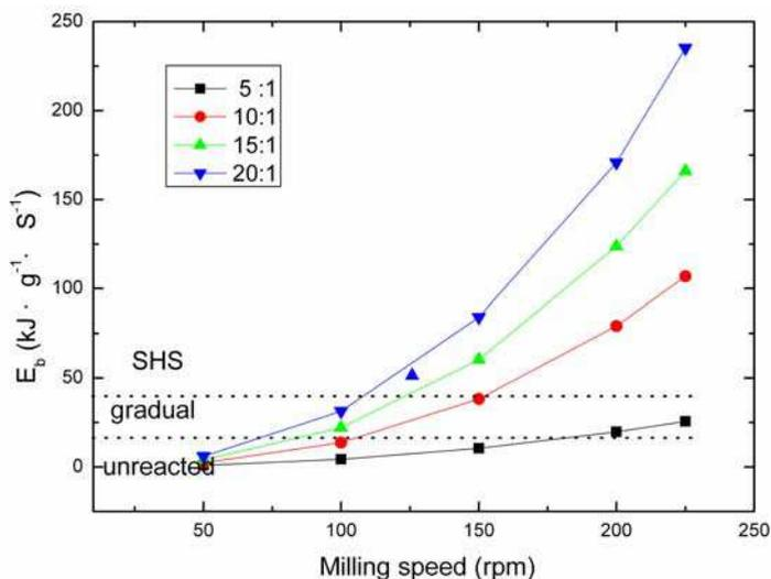
Fig. 3. Milling map of WC/MgO at different conditions
