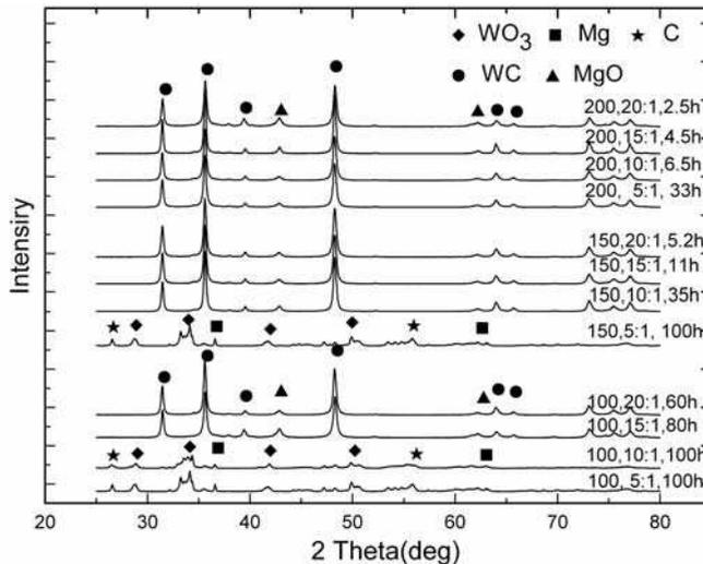
Fig. 2. XRD patterns of powders milled at different milling speed and ball-to-powder weight ratio for different milling time
