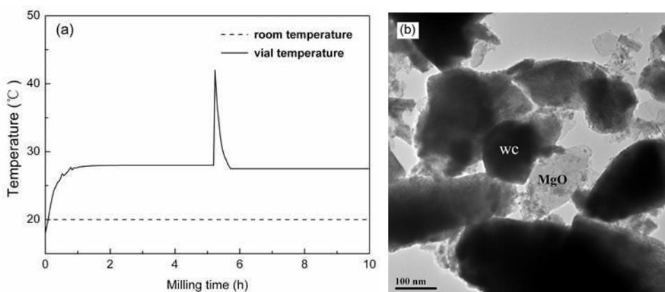
Fig. 8. (a) Temperature variation of milling vial during milling for reaction (1) and (b) the corresponding TEM micrograph
