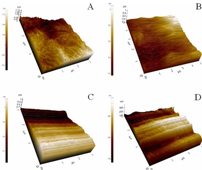
Fig. 6. AFM images of sample (A) PEEK, (B) PEEK/pristine MWCNT, (C) PEEK/ZrO<sub>2</sub> coated MWCNT by isothermal process, (D) PEEK/ZrO<sub>2</sub> coated MWCNT by chemical process
