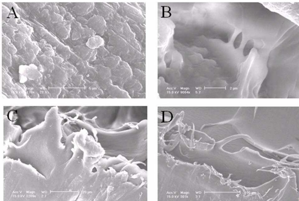
Fig. 7. FESEM images of composite (A) PEEK, (B) PEEK/pristine MWCNT, (C) PEEK/ZrO<sub>2</sub> coated MWCNT by isothermal process, (D) PEEK/ZrO<sub>2</sub> coated MWCNT by chemical process
