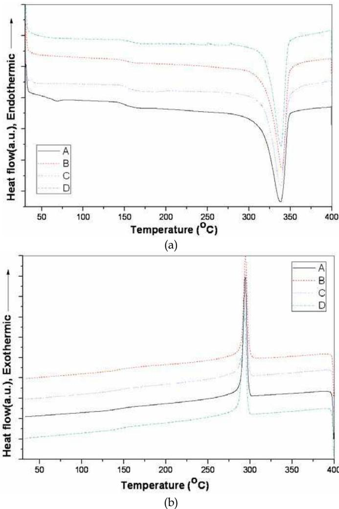
Fig. 4. (a) Endotherm and (b) exotherm result of the composites (A) PEEK. (B) PEEK/pristine MWCNT, (C) PEEK/ZrO<sub>2</sub> coated MWCNT by isothermal process, (D) PEEK/ZrO<sub>2</sub> coated MWCNT by chemical process
