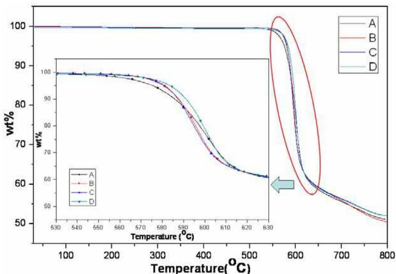
Fig. 5. TGA result of the composites (A) PEEK. (B) PEEK/pristine MWCNT, (C) PEEK/ZrO<sub>2</sub> coated MWCNT by isothermal process, (D) PEEK/ZrO<sub>2</sub> coated MWCNT by chemical process
