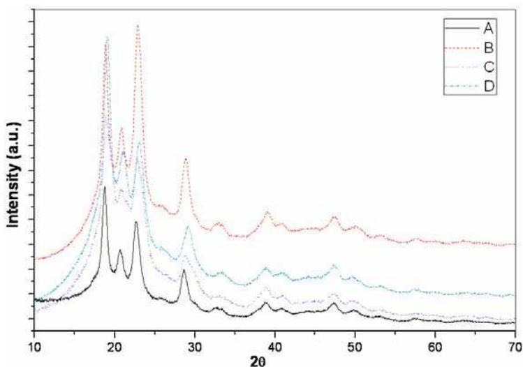
Fig. 2. XRD result of sample (A) PEEK, (B) PEEK/pristine MWCNT, (C) PEEK/ZrO<sub>2</sub> coated MWCNT by isothermal process, (D) PEEK/ZrO<sub>2</sub> coated MWCNT by chemical process
