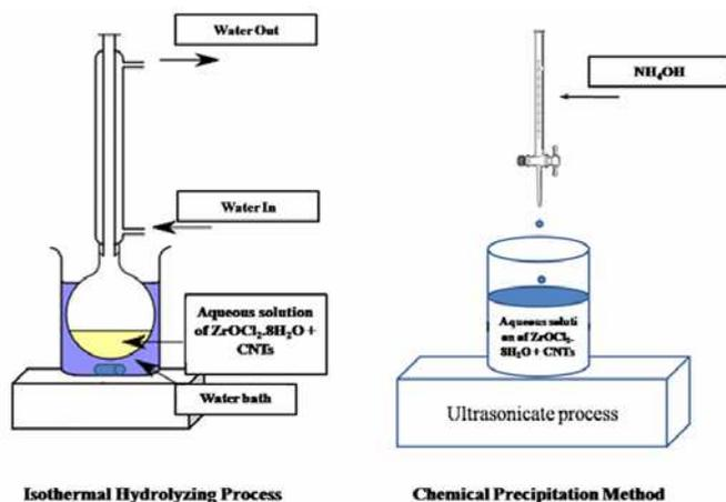
Fig. 1. A diagram of hydrolysis method and chemical precipitation methods for prepared nanocomposites
