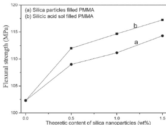
Fig. 20. Flexural strength of different PMMA nanocomposites [14].
