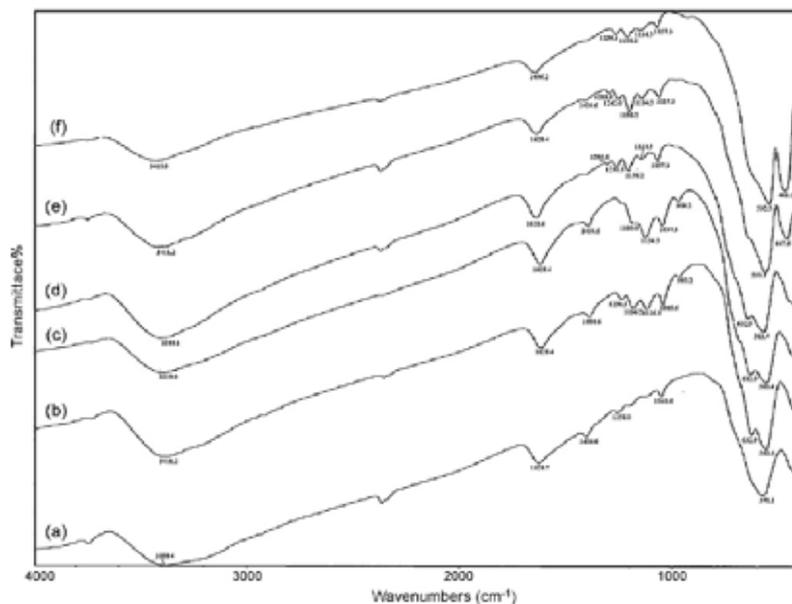
Fig. 18. IR spectra of pure  $\text{Fe}_3\text{O}_4$  nanoparticles at room temperature (a) and calcined at  $150^\circ\text{C}$  (b),  $250^\circ\text{C}$  (c),  $350^\circ\text{C}$  (d),  $450^\circ\text{C}$  (e),  $550^\circ\text{C}$  (f) for 2 h in the atmosphere [28].
