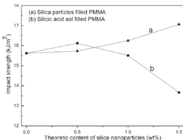
Fig. 19. Impact strength of different PMMA nanocomposites [14].
