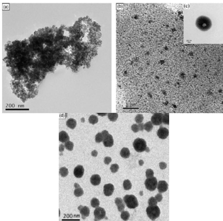
Fig. 13. TEM images of (a) bare  $\text{Fe}_3\text{O}_4$  nanoparticles; (b) CS-PAA particles; (c) magnified CS-PAA particles; (d)  $\text{Fe}_3\text{O}_4$  nanoparticles synthesized by CS-PAA template [23].
