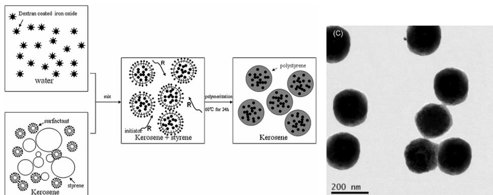
Fig. 15. The procedure for preparation of  $\text{Fe}_3\text{O}_4/\text{PS}$  composite particles by inverse emulsion polymerization (left); TEM images of  $\text{Fe}_3\text{O}_4/\text{PS}$  composite microspheres (right) [26].
