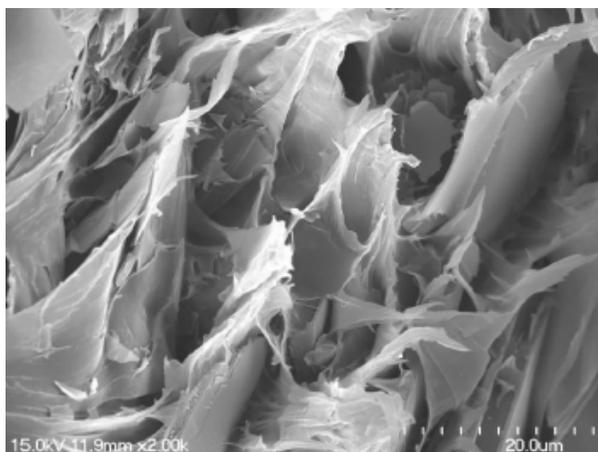
Fig. 16. SEM of the fracture of EGP/LEDP composites (35% EGP, no phase separation) [27].
