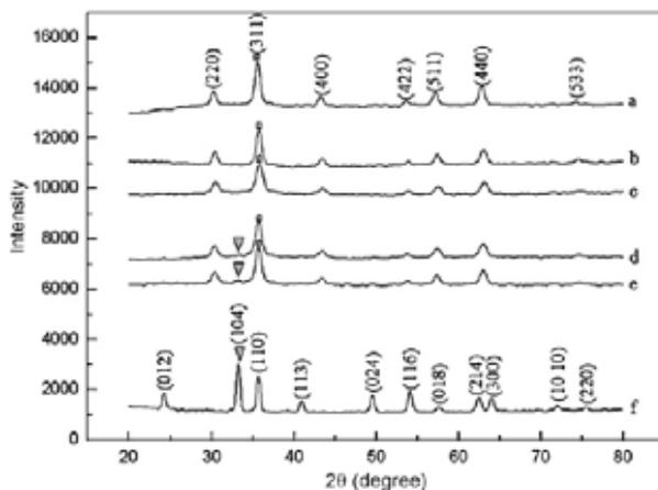
Fig. 17. XRD patterns of pure  $\text{Fe}_3\text{O}_4$  nanoparticles at room temperature (a) and calcined at  $150^\circ\text{C}$  (b),  $250^\circ\text{C}$  (c),  $350^\circ\text{C}$  (d),  $450^\circ\text{C}$  (e),  $550^\circ\text{C}$  (f) for 2 h in the atmosphere [28].
