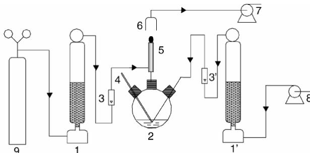
Fig. 1. Experimental flow diagram for synthesizing  $\text{TiO}_2$  nanoparticles using LPG/air flame. (1 and 1': Dryer, 2:  $\text{TiCl}_4$  evaporator, 3 and 3': rotameters, 4: thermometer, 5: combustor, 6: filter, 7: circulating-water vacuum pump, 8: air compressor, 9: LPG cylinder) [1].
