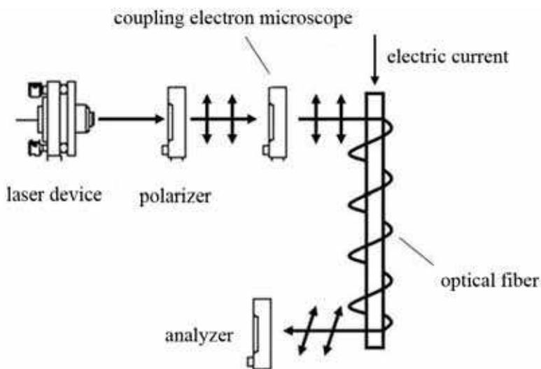
Fig. 21. The structure of a current sensor using optical fiber.
