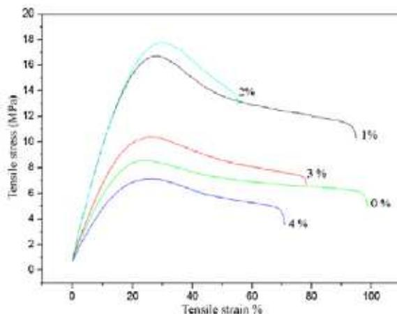
Fig. 14. Tensile stress-strain curves of different PU films [24].
