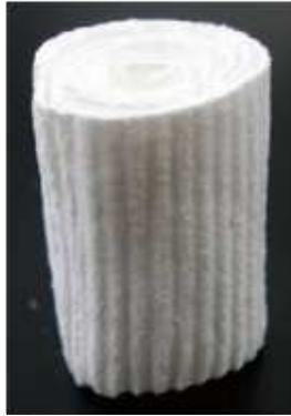
Fig. 8. Unidirectional porous HAp/Col bone-like nanocomposite.
