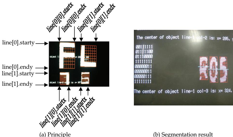
Fig. 2. The classical image segmentation algorithm
