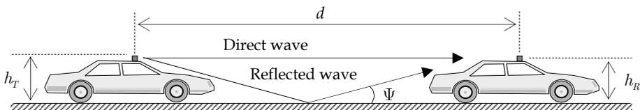
Fig. 5. Geometry for the two-ray propagation model
