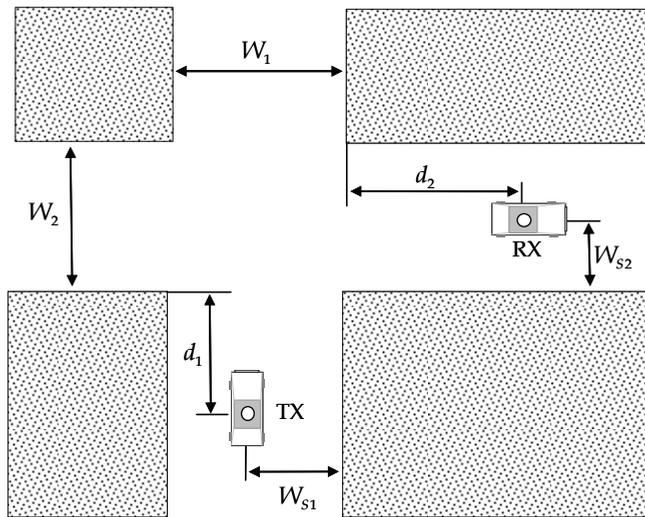
Fig. 8. Geometry of the Kangaku University path loss model for NLOS conditions (Sai et al., 2009)
