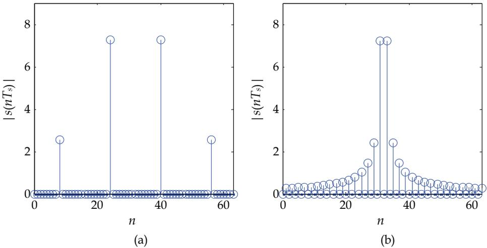
Fig. 3. Samples of the envelope of an MC-CDMA signal for a single user and different WH codes. (a)  $k=2$ . (b)  $k=16$
