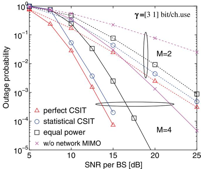
Fig. 2. Outage probability versus signal-to-noise ratio for  $M \in \{2, 4\}$  antennas per base station.
