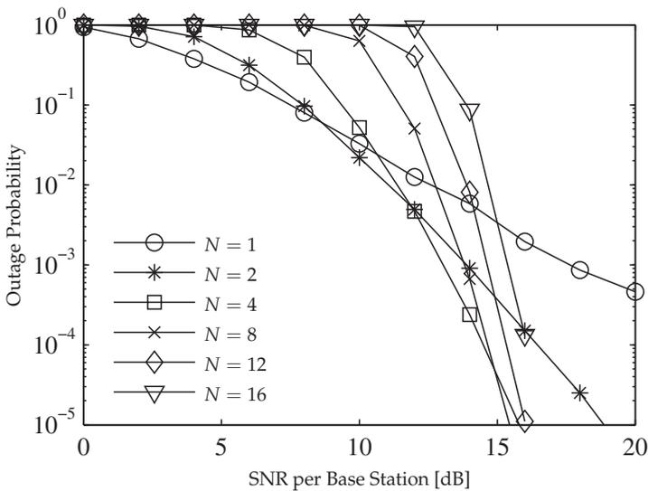
Fig. 8. Outage probability as a function of SNR
