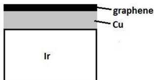
Fig. 24. Schematic structure of the layer transformation for the system Ir(111) - graphene - Cu: (a) - Cu film of  $\sim 2$  ML thickness is deposited upon graphene on Ir(111) ( $T=3000\text{K}$ ); (b) - the same layer after annealing at  $1200\text{K}$ .
