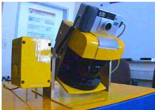
Fig. 15. A 3D laser range finder for autonomous mobile robots. The servo is mounted at the left side. A camera on top is used to get texture images for the realistic appearances of a 3D scene (Surmann et al. 2001)
