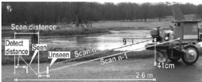
Fig. 14. The robot used in the experiments has a laser scanner at a height of 41 cm looking down in an angle of \theta_L = 9^\circ . The road is therefore detected at 2.6 m. The position of the last scan (scan n - 1 ) is shown to illustrate the largest undetected obstacle. The unseen object is not detected in scan n - 1 and is too short to be seen by scan n
