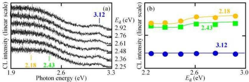
Fig. 5. (a) CL spectra after the illumination of a light with the photon energy  $E_{ill}$  as in Fig. 4. (b) The CL intensity at 3.12, 2.43, or 2.18 eV vs  $E_{ill}$ . (Ohno et al, 2009b). Copyright Wiley-VCH Verlag GmbH & Co. KGaA. Reproduced with permission
