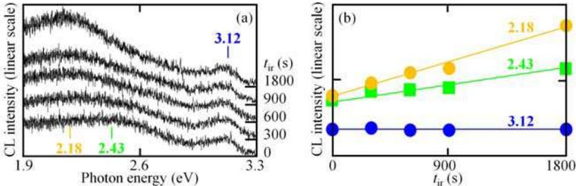
Fig. 6. (a) CL spectra after the irradiation of electrons, with flux of  $5 \times 10^{17} e \text{ mm}^{-2} \text{ s}^{-1}$  at temperature of 120 K, for the irradiation time  $t_{ir}$ . (b) The CL intensity at 3.12, 2.43, or 2.18 eV vs  $t_{ir}$ . (Ohno et al, 2009b). Copyright Wiley-VCH Verlag GmbH & Co. KGaA. Reproduced with permission
