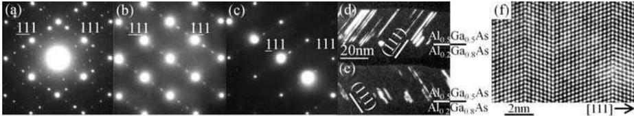
Fig. 9. Diffraction patterns of a twinned  $\text{Al}_{0.5}\text{Ga}_{0.5}\text{As}$  epilayer taking along (a)  $[110]$ , (b)  $[011]$ , and (c) nearly  $[011]$ . TEM images taking with a twin spot at (d)  $1/3, 1/3, 5/3$  and (e)  $1/3, 1/3, 5/3$ . (f) A high-resolution TEM image of twin boundaries. (Ohno et al, 2007b)
