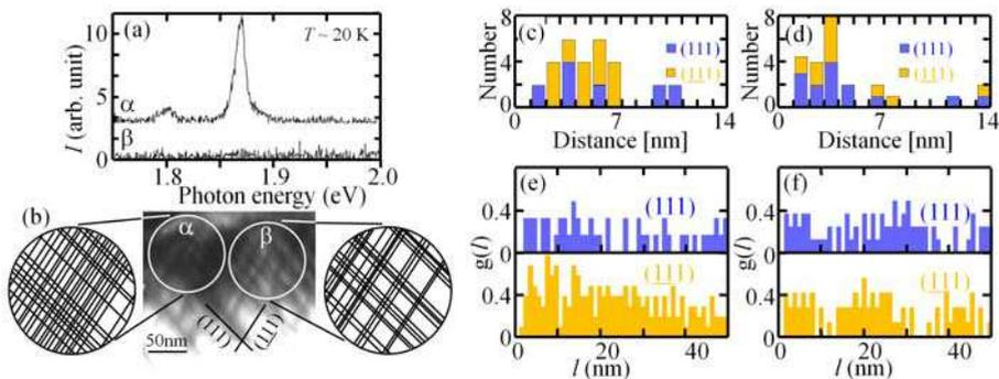
Fig. 11. (a) CL spectra obtained from the encircled areas  $\alpha$  and  $\beta$  in (b) [the insets in (b) show the locations of the boundaries in the areas]. (c) or (d), respectively, shows the histogram of the intervals between the nearest-neighbor boundaries in  $\alpha$  or  $\beta$ . (e) or (f), respectively, shows the distribution function of boundaries in  $\alpha$  or  $\beta$ . (Ohno, 2010b)
