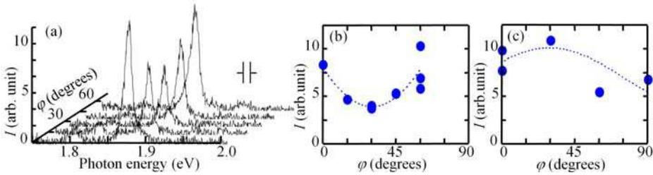
Fig. 12. (a) Polarized CL spectra for different  $\phi$  obtained from  $\alpha$  in Fig. 11b. The experimental setup is similar to that in Fig. 10a, and the specimen is set so that the z axis is parallel to [001]. The CL intensity  $I$  vs  $\phi$ ; the z axis is parallel to (b) [001] or (c) [110] (Ohno et al, 2007b)
