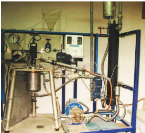
Fig. 2. The esterification reactor used for the experiments.
