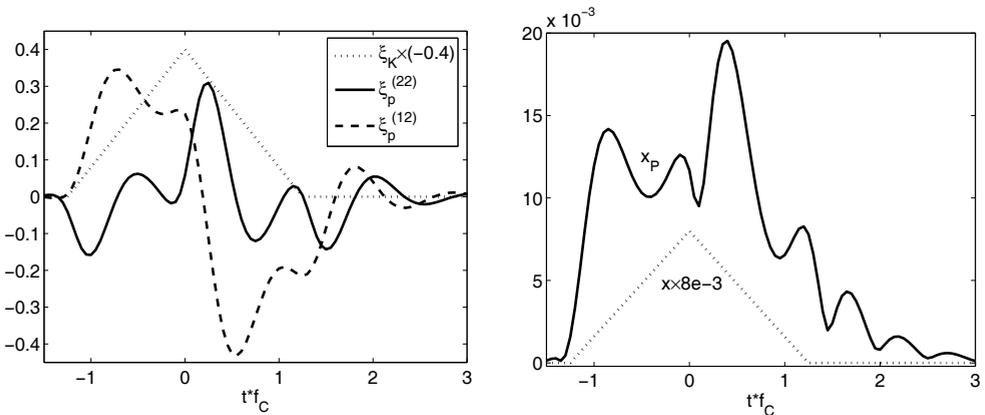
Fig. 6. Left: Sensitivity signals  $\xi$  for the amplification  $K$  and the two pole projections  $\rho_1, \rho_2$ , obtained by digital filtering of the corrected output shown in Fig. 3 (right). Right: Resulting confidence interval half-width  $x_p$ . For comparison, the rescaled input signal is shown (dotted).
