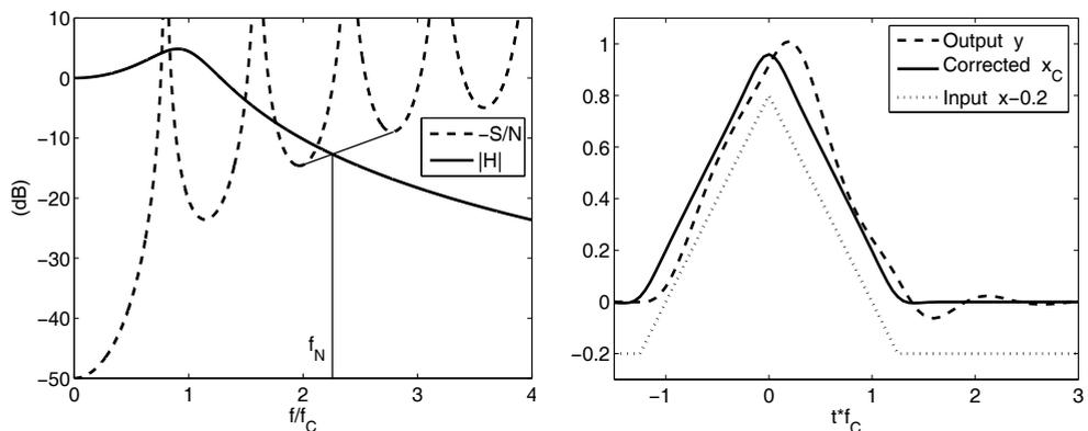
Fig. 3. Left: Signal to noise ratio ( $S/N$ ) for the input signal (Fig. 2) and amplification  $|H|$  of the measurement system, for determining the cut-off frequency  $f_N$  of the noise filter. Right: The output and the corrected output. The input signal is indicated (displaced for clarity).
