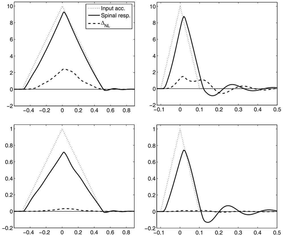
Fig. 11. Lumbar spine response and its difference to linearized response  $\Delta_{NL}$ , for various pulse acceleration amplitudes  $A$  and widths  $T$ :  $A = 10 m/s^2$  (top),  $A = 1 m/s^2$  (bottom),  $T = 1 s$  (left), and  $T = 0.2 s$  (right). The units are  $m/s^2$  (vertical) and  $s$  (horizontal).
