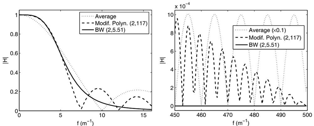
Fig. 13. Magnitude of frequency response of smoothing filters, in the low (left) and high (right) frequency range: the averaging filter (right:  $\times 0.1$ ), the modified square polynomial 117-tap FIR filter, and the proposed second order Butterworth filter (BW) with cross-over frequency  $5.5 \text{ m}^{-1}$ .
