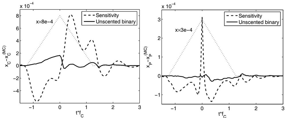
Fig. 8. The errors of the center  $x_C$  (left) and the half-width  $x_P$  (right) of the confidence interval of the correction, for the sensitivity analysis (section 3.3.1) and the method of unscented binary sampling (section 3.3.2). The errors are estimated with random sampling of  $10^6$  correction filters. For comparison, the rescaled input signal is shown (dotted).
