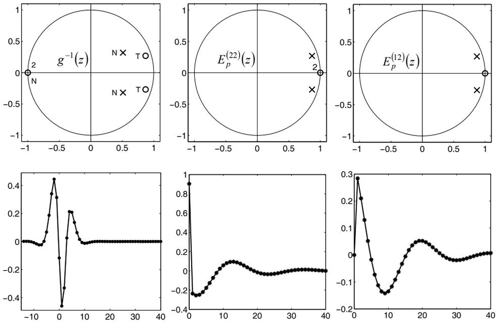
Fig. 5. Poles (x) and zeros (o) (top) and impulse responses (bottom) of the correction  $g^{-1}(z)$  (left) and digital sensitivity filters  $E_p^{(22)}(z)$  (middle) and  $E_p^{(12)}(z)$  (right) for the two projections  $\rho_1$  and  $\rho_2$ , respectively.
