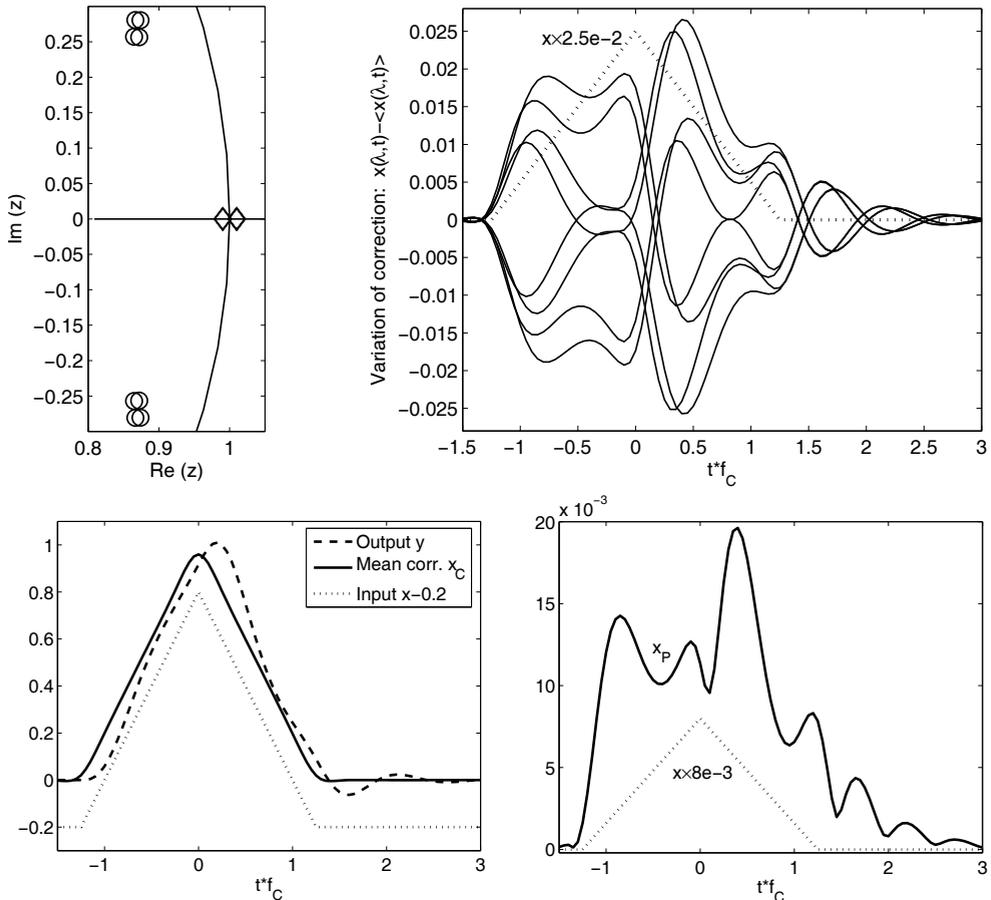
Fig. 7. Top left: Poles and zeros of the eight sampled digital correction filters, excluding the fixed noise filter. The static gains ( $\diamond$ ) are displayed on the real  $z$ -axis (close to  $z=1$ ). Top right: The variation of all corrections from their mean. Bottom: Center  $x_C$  (left) and half-width  $x_p$  (right) of the confidence interval for the correction. The (rescaled/displaced) input signal of the measurement system is shown (dotted) for comparison.
