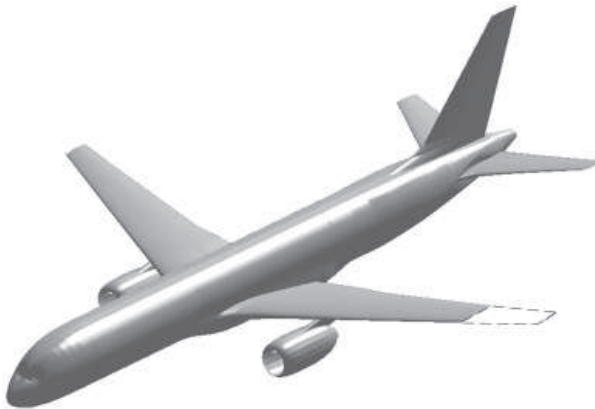
Fig. 2. Left Wing Damaged Generic Transport Model
