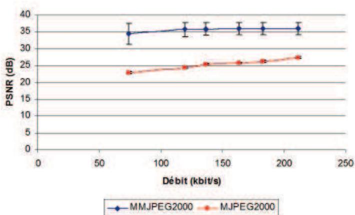
Fig. 7. MMJPEG2000 vs MJPEG2000 : Survey sequence
