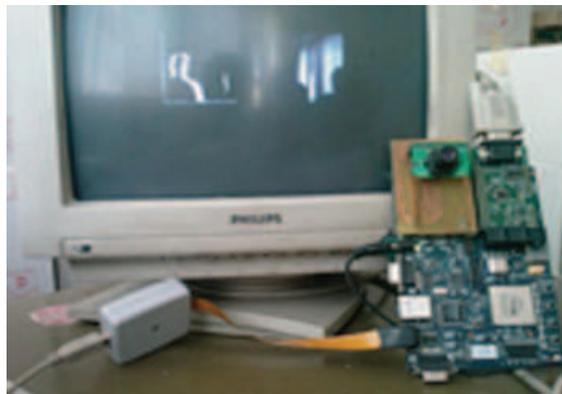
Fig. 14. Motion detection experimental prototype
