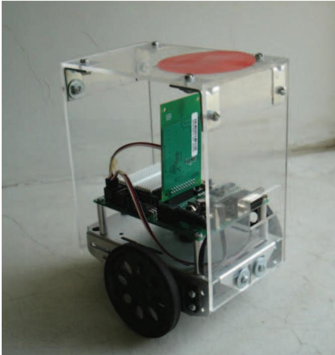
Fig. 5. Mobile Robot Prototype
