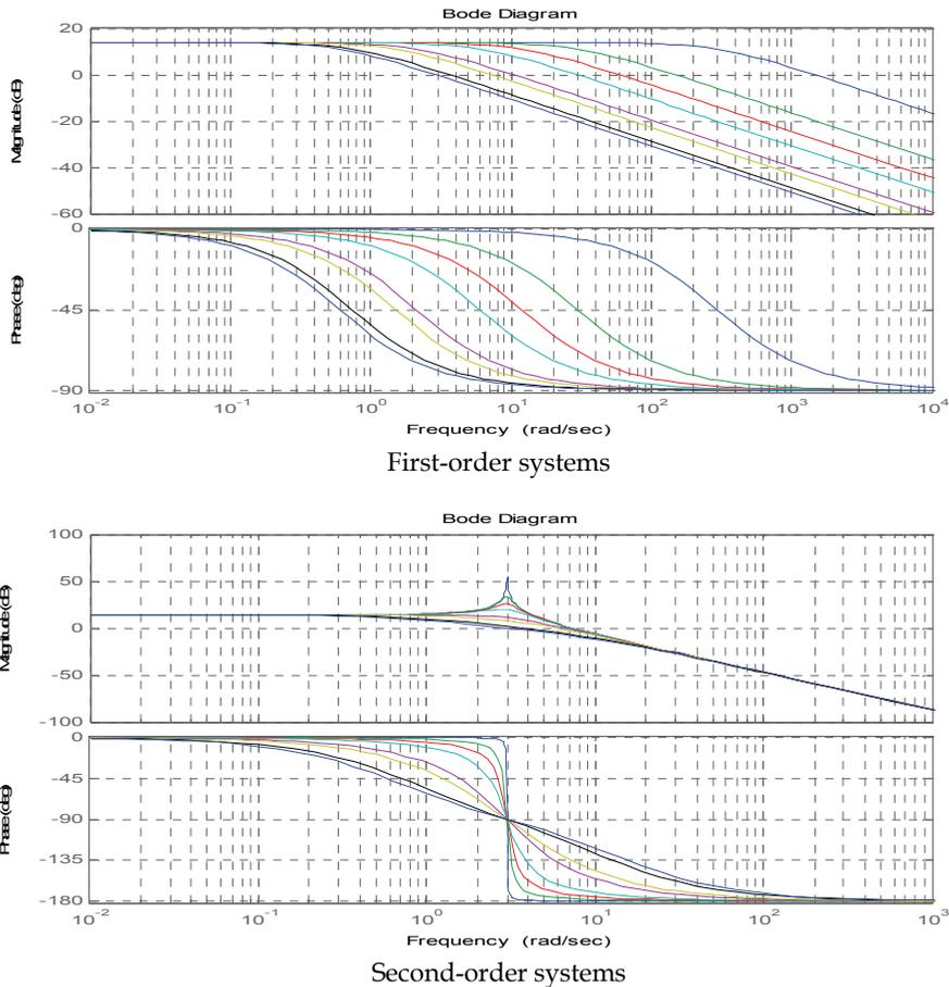
Fig. 5. Bode diagram of first and second-order systems
