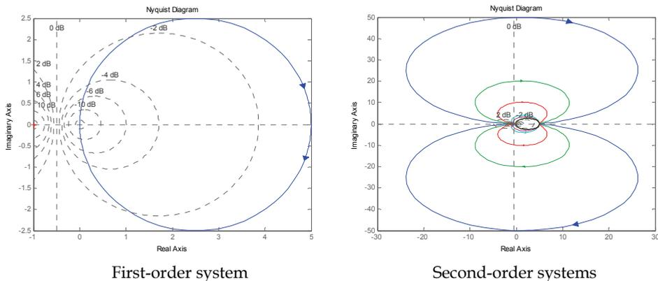
Fig. 4. Nyquist plots of linear transfer elements
