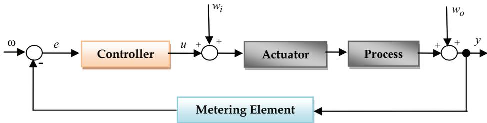
Fig. 2. Elements of a control loop
