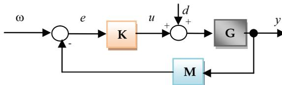
Fig. 9. Closed-loop system
