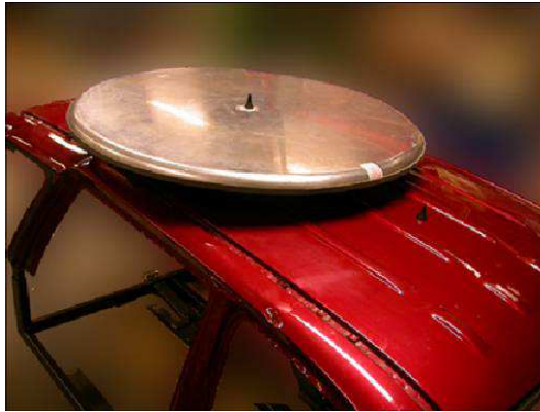
Fig. 4. Photograph of the measurement antenna solution with an extra disc added on top of the car
