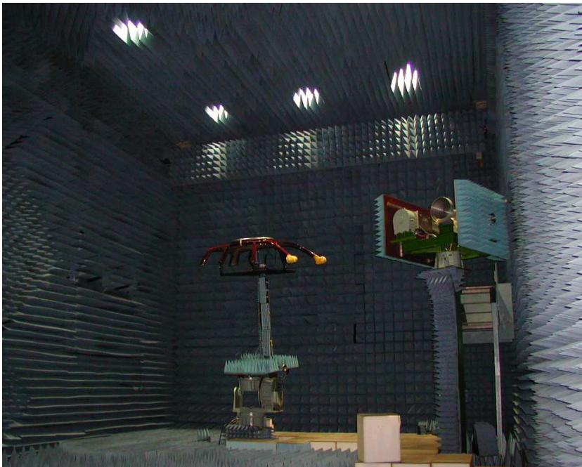
Fig. 5. The monopole antenna during verification measurements at Allgon's (today Powerwave) compact range in Stockholm Sweden. The monopole and the disc ground plane are mounted on the roof from a chassis of the same car as in the actual Swedish 3G verification measurements
