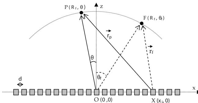
Fig. 1. Geometry for computing the focusing delays.
