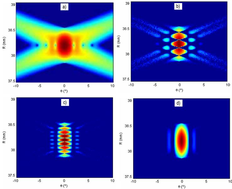
Fig. 12. Images of a point reflector obtained with conventional beamforming (a) and after processing with *FCF* (b), *FCS* (c) and *FCC* (d). Dynamic range 70 dB;  $N=64$  elements,  $d=\lambda/2$ ,  $f_s = 5$  MHz,  $BW=0.5$  and  $SNR = 60$  dB per channel.
