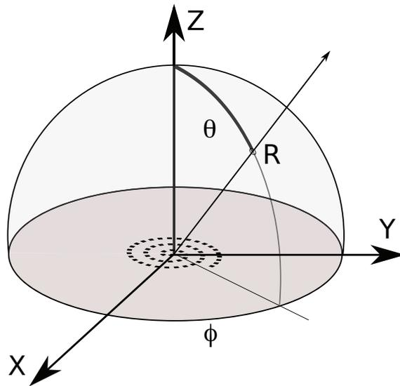
Fig. 1. Coordinate system used to compute de array beampattern. The array is located in the XY plane ( $\theta = 0$ ) and the field is computed in a hemisphere, defined for narrowband by  $(\theta, \phi)$  and for wideband by  $(R, \theta, \phi)$ .
