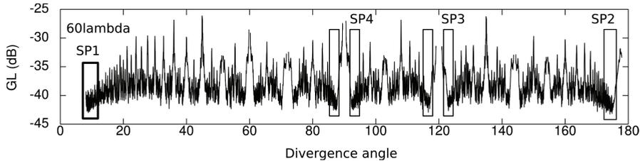
Fig. 5. Grating lobe levels vs the divergence angle, for wideband response (two ways,  $\Delta\alpha = 0^\circ$ ,  $\lambda=0.5\text{mm}$ ,  $\text{BW}=60\%$ ). Rectangles show the location of the best apertures.
