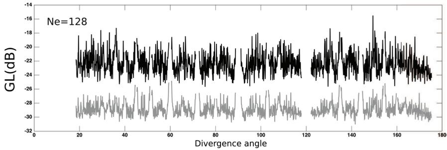
Fig. 4. Narrowband Grating lobe distribution per divergence angle. Black line represents the echo-pulse response if  $\Delta\alpha = 0^\circ$ ; the gray line represents the echo-pulse response of the better case obtained when  $\Delta\alpha > 0^\circ$ .
