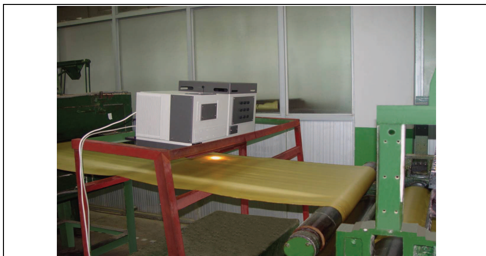
Fig. 7. Application of NIR for quality monitoring in the production of glass/phenolic prepreg cloth
