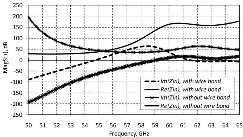
Fig. 3.4. Real and imaginary components of input impedance (antenna with and without wire bond).
