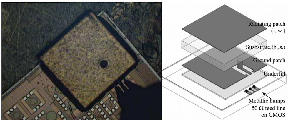
Fig. 2.1. Patch antenna structure on CMOS chip (photograph and geometry of fabricated antenna). (Parameters:  $l=1.65\text{mm}$ ,  $w=1.67\text{mm}$ ,  $\epsilon_r=2.2$ ,  $y'=0.435\text{mm}$ ,  $h_s=0.254\text{mm}$ )
