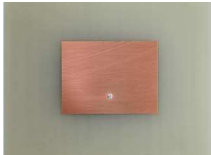
Fig. 19. Photo of the LP microstrip antenna prototype.
