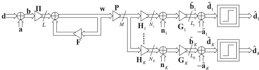
Fig. 3. Equivalent linear representation of THP in Fig. 2.
