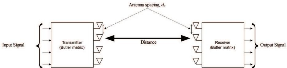
Fig. 3. The Concept of RF MIMO Front End Systems Measurement
