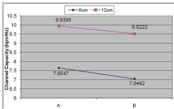
Fig. 5. Average Channel Capacity for Normal Configuration
