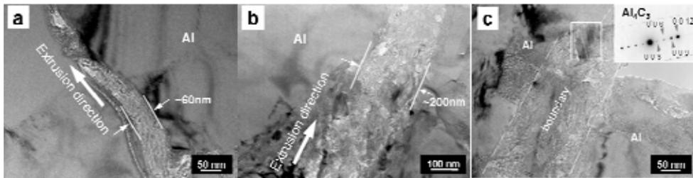
Fig. 6. TEM micrographs of (a) the extruded Al-1vol% CNT composite and (b) the extruded Al-5vol% CNT composite. (c) The implanted  $Al_4C_3$  between the Al matrix and CNT in the Al-5vol% CNT composite (Kwon et al., 2009). The inset shows the SADP of the  $Al_4C_3$ .
