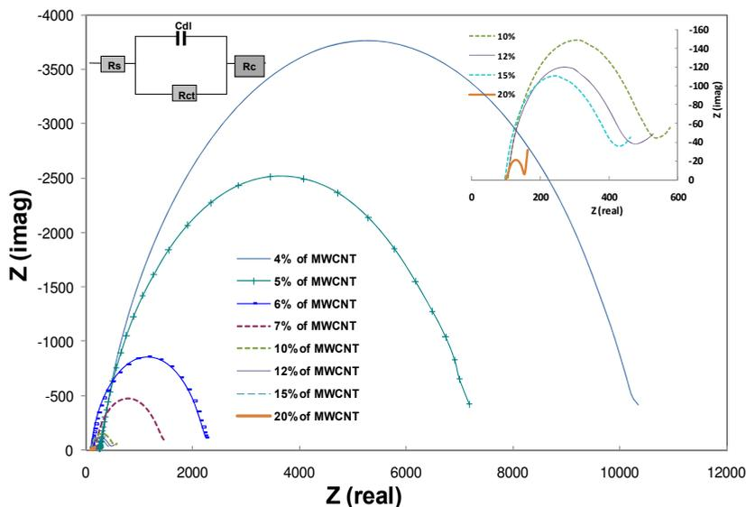
Fig. 9. Impedance spectra for different MWCNT loading electrodes in the presence of  $\text{Fe}(\text{CN})_6^{3-/4-}$ . The insets in the figure show the equivalent circuit used for the impedance spectra fitting and a zoom of the low impedance composite electrodes. Reproduced from Ref. (Olivé-Monllau et al., 2010) with permission. Copyright, 2010, Elsevier.
