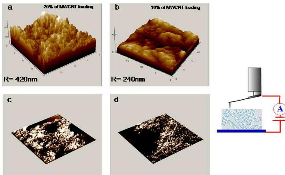
Fig. 4. Topographical AFM images with their corresponding conductivity mappings for 20% of CNT loading (a,c) and 10% of CNT loading (b,d). The x-axis, y-axis and z-axis units are  $\mu\text{m}$ ,  $\mu\text{m}$  and nm respectively. Scheme of a C-AFM set-up. Adapted from Ref. (Olivé-Monllau et al., 2010) with permission. Copyright, 2010, Elsevier.
