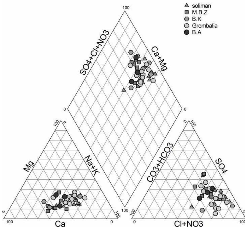
Fig. 3. Piper diagram of the Grombalia unconfined aquifer
