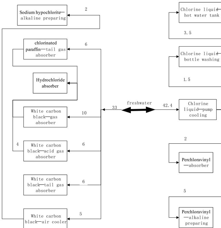
Fig. 13. Water reuse scheme in plant 2
