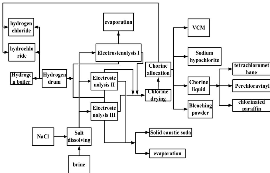
Fig. 1. Schematic flow sheet of the chlor-alkali complex
