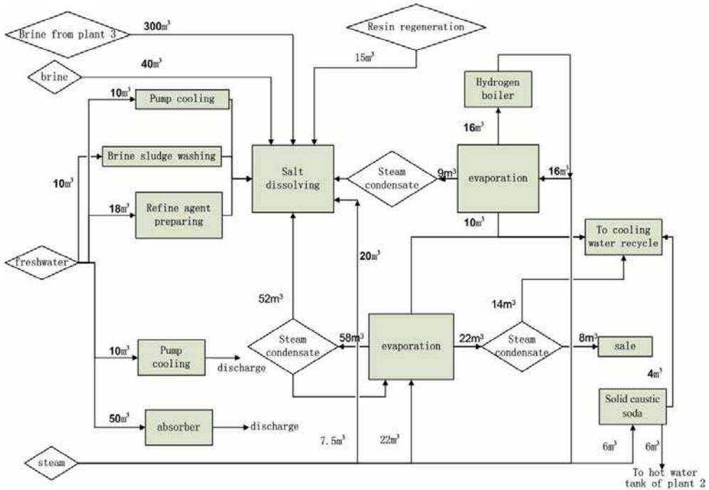
Fig. 2. Balanced water system of plant 1
