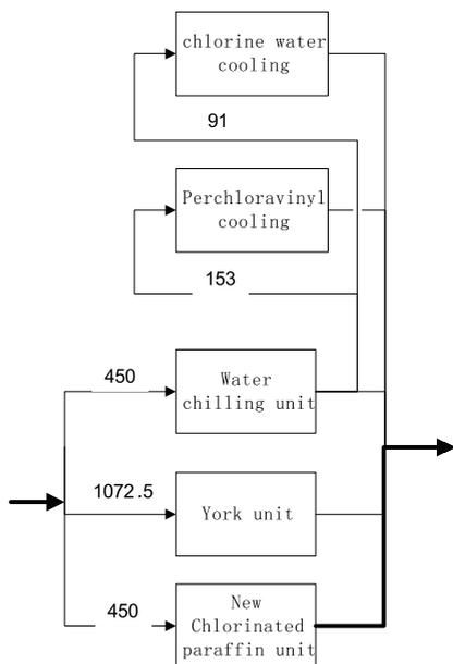
Fig. 10. Cooling water system retrofit solution 1
