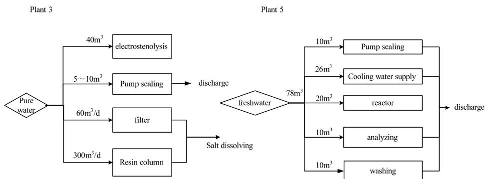
Fig. 4. Balanced water system of plant 3 and 5
