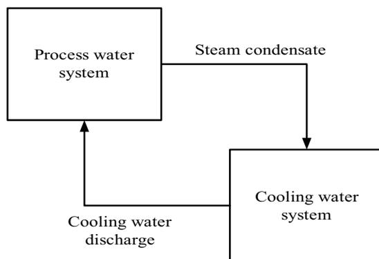
Fig. 5. Schematic figure of the total water system
