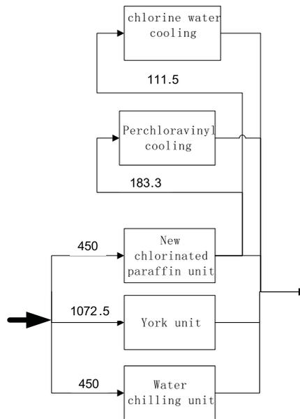
Fig. 11. Cooling water system retrofit solution 2
