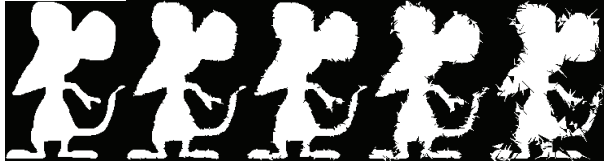
Fig. 9. Examples of noisy shapes from a model in MPEG-7 CE-Shape-1. From left to right, the original and the resulting noised shapes at an SNR of 30dB, 25dB, 20dB and 15dB.
