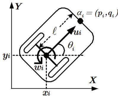
Fig. 8. Kinematic model of unicycles
