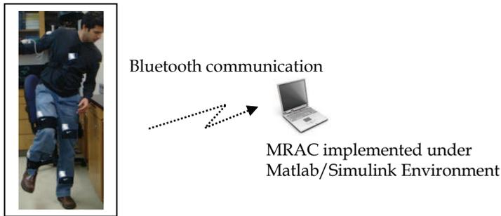
Fig. 4. Nintendo Wiimotes based human motion capturing system
