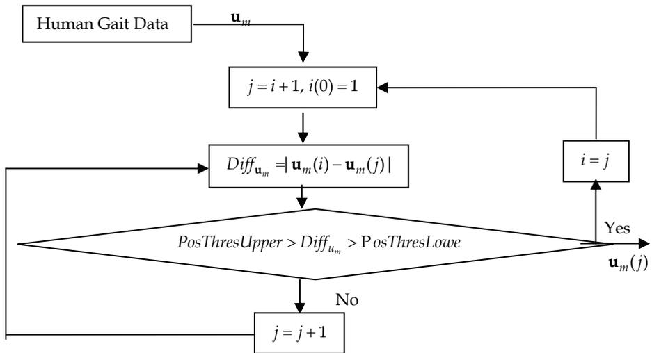
Fig. 5. Filter algorithm for human motion data
