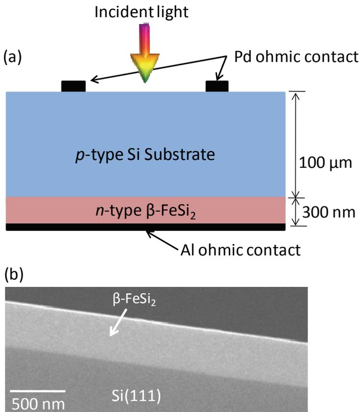
Fig. 6. (a) Schematic illustration of an n-type  $\beta\text{-FeSi}_2$  (300 nm)/p-type Si (100  $\mu\text{m}$ ) heterojunction photodiode with Pd and Al electrodes on top (Si) and bottom ( $\beta\text{-FeSi}_2$ ) surfaces, respectively. (b) Cross-sectional SEM image of  $\beta\text{-FeSi}_2$  film deposited on Si(111) substrate.
