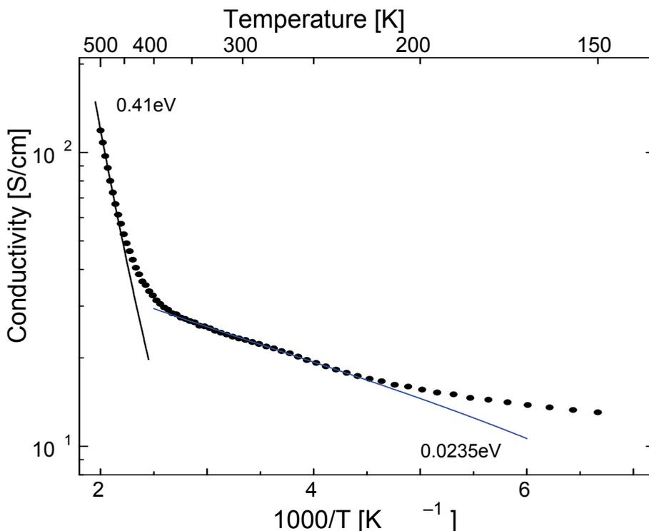
Fig. 5. Temperature dependence of the electric conductivity of the  $\beta$ -FeSi<sub>2</sub> film.
