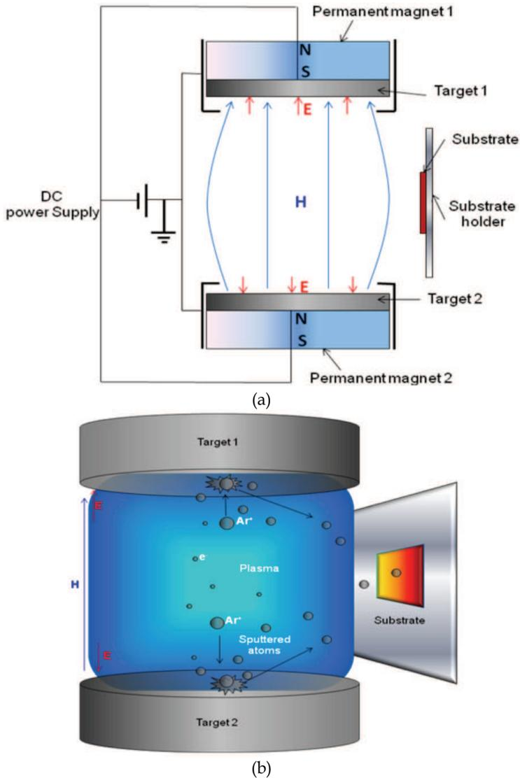
Fig. 1. Illustrations of; (a) FTDCS configuration, and (b) sputtering mechanism in FTDCS apparatus
