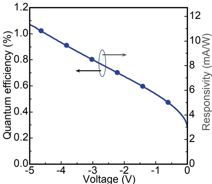
Fig. 9. Quantum efficiency and current responsivity of  $\beta$ -FeSi<sub>2</sub>/Si heterojunction photodiode plotted against reverse bias under illumination with a 6 mW, 1.31  $\mu$ m.
