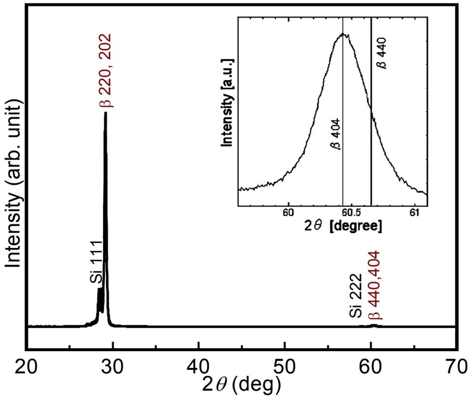
Fig. 2. X-ray diffraction pattern of the  $\beta$ -FeSi<sub>2</sub> thin film measured by a  $2\theta$ - $\theta$  method. The inset is the extension of  $\beta$ -404, 440 peaks.
