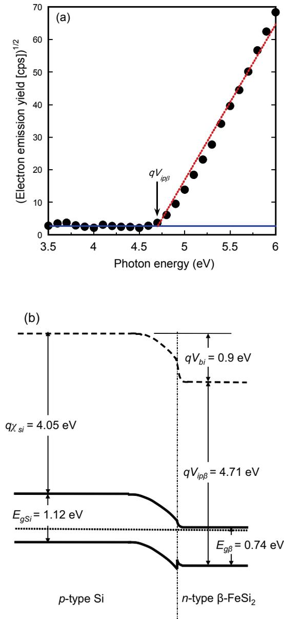
Fig. 4. (a) Photoelectron spectrum of a  $\beta$ -FeSi<sub>2</sub> film, wherein the threshold value of the photon energy corresponds to the ionization potential and (b) the energy band diagram of n-type  $\beta$ -FeSi<sub>2</sub>/p-type Si heterojunction.
