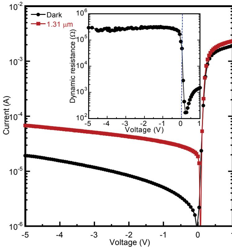
Fig. 7. *I-V* characteristics measured in the dark and under illumination with a 6 mW, 1.31  $\mu\text{m}$  LD at room temperature. The inset shows the dynamic junction resistances deduced from the *I-V* characteristics.
