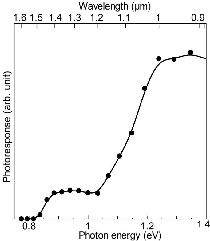
Fig. 8. Photoresponse spectrum of  $\beta$ -FeSi<sub>2</sub>/Si heterojunction photodiode measured in the NIR range at zero bias and room temperature.
