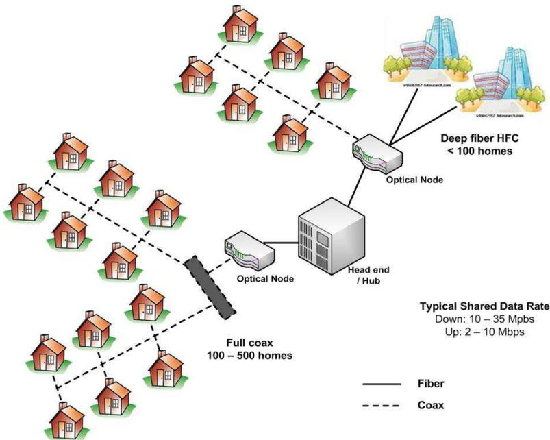
Fig. 4. Cable TV, Hybrid Fiber Coax (HFC) architectures.
