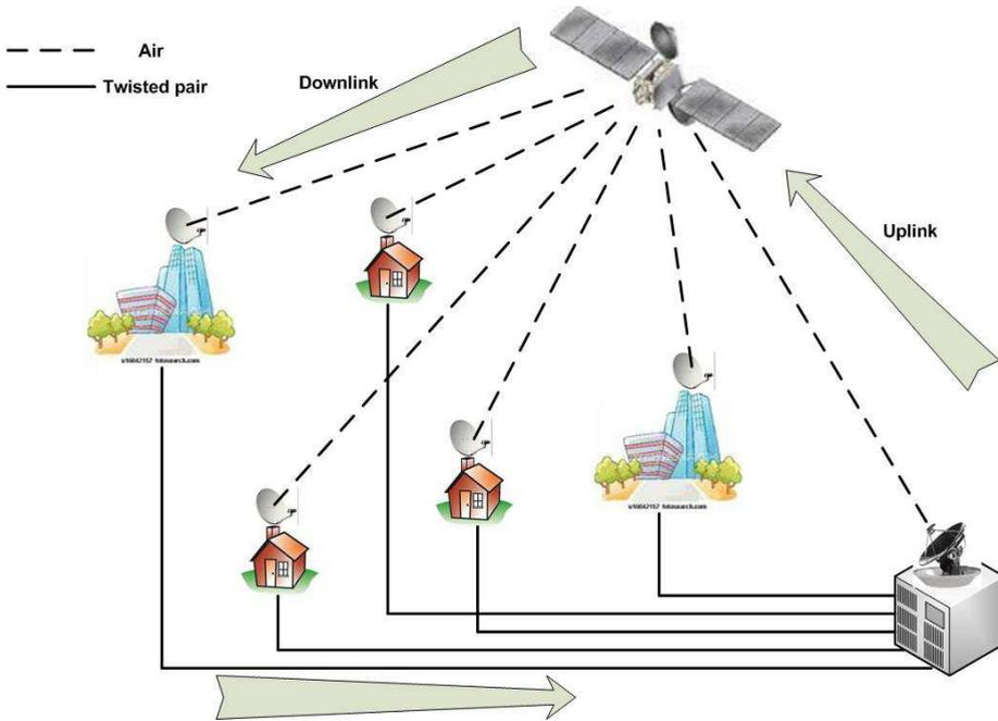
Fig. 7. Direct Broadcast Satellite (DBS) network architecture.
