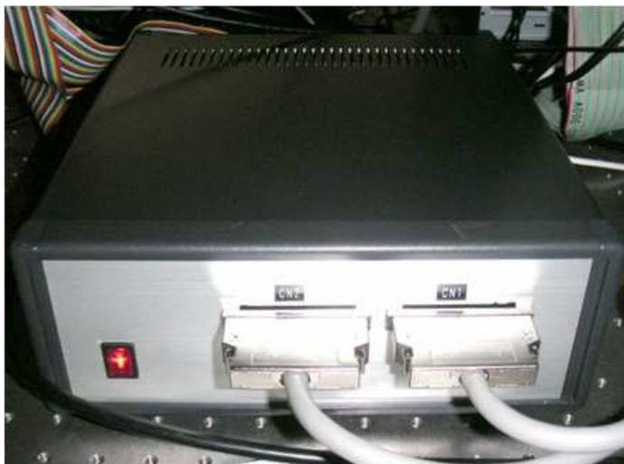
Fig. 6. Electrical part of the compact laser communication transceiver
