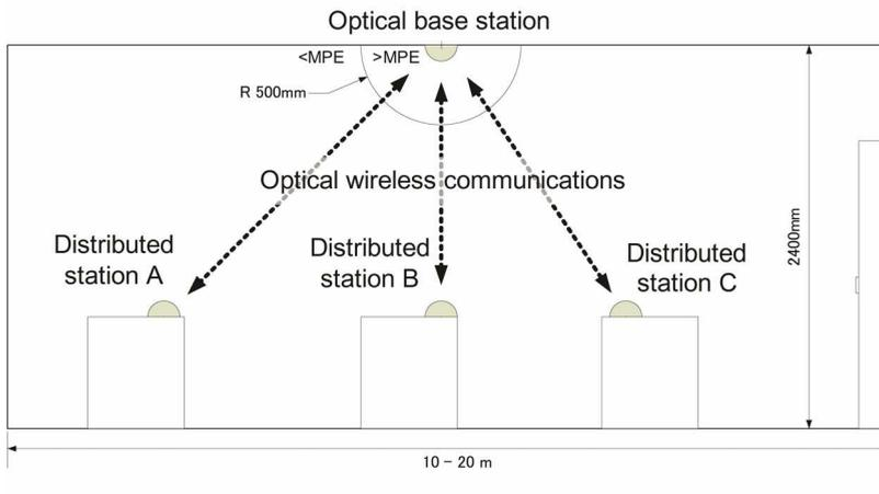
Fig. 7. Optical base station and distributed optical station layout
