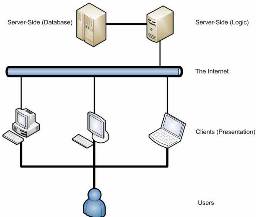
Fig. 1. Three-tier system architecture used to design *CropWaterUse*
