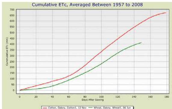
Fig. 6. Calculated average daily cumulative crop evapotranspiration as a function of days after sowing for cotton and wheat at Oakey
