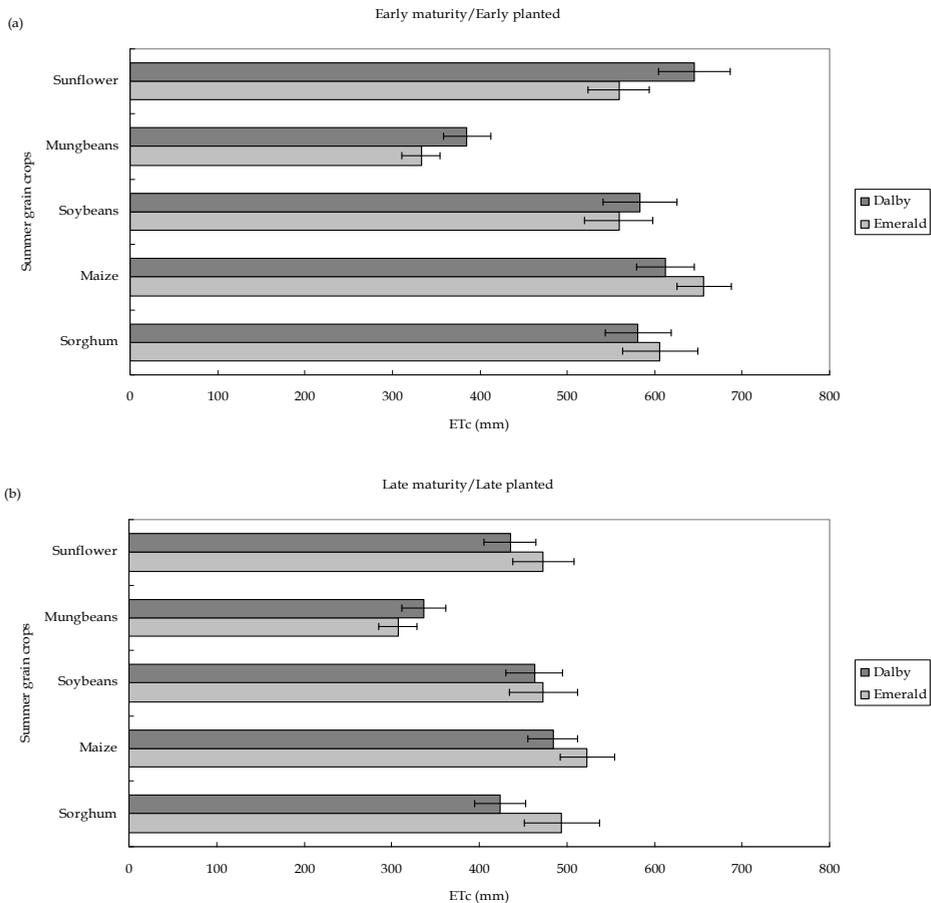
Fig. 14. Range of crop evapotranspiration (ETc) as estimated by the *CropWaterUse* tool using historical weather data (1957-2008) for “fully irrigated” sunflower, mungbeans, soybeans, maize and sorghum for various scenarios (a) early planting, early maturing varieties, and (b) late planting, late maturing varieties in cooler (at Dalby) and hotter (at Emerald) climatic conditions in Queensland. Bar indicates +/- standard deviation
