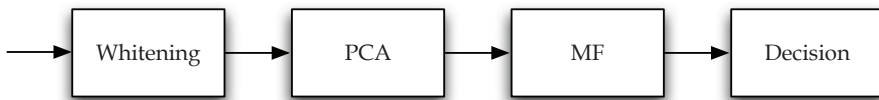
Fig. 7. Block diagram of the matched filter for stochastic signals considering colored noise.
