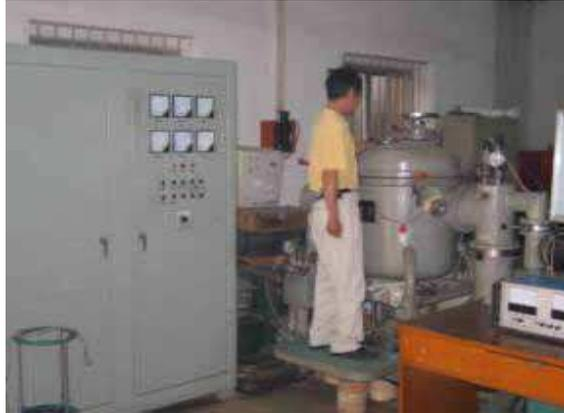
Fig. 20. Medium frequency induction melting furnace
